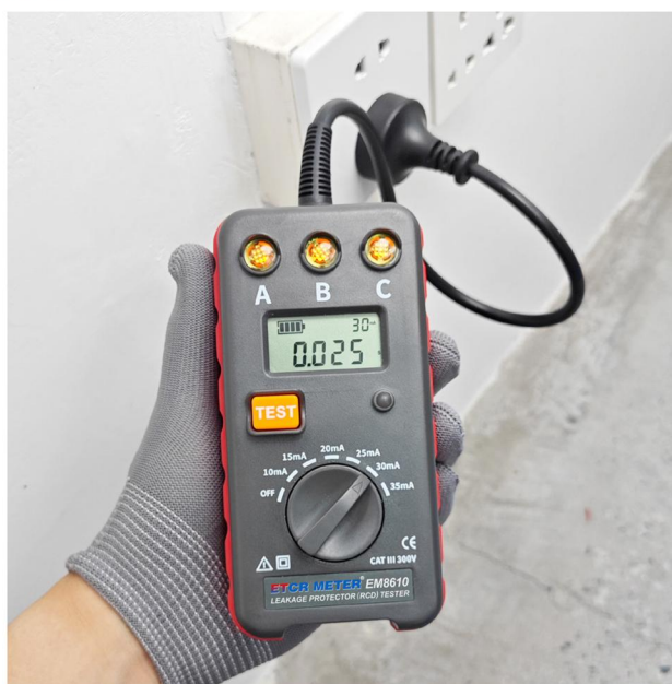
< Socket Leakage Test >
